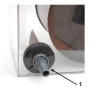
If the Rollermat is supplied with water by a pump, the maximum flow is 2700l/h (e.g. River 2700). The water inlet has to be reduced by a reduction fitting to a  $\frac{3}{4}$ " hose connector. This connections should be glued.
