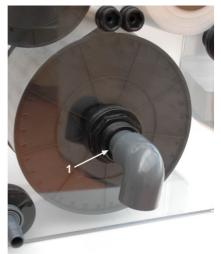
The water outlet may not be reduced. A 40 mm PVC pipe should be presses into the tank union. From here a PVC pipe can be directed to the filter sump or pond. The pipe should not be glued into the tank union. If it is glued, the Rollermat cannot not be disassembled.
