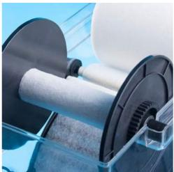
The fleece is transported from the releasing roll to the accepting roll. The rolls are driven by gear wheels.
