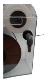
The emergency overflow is a 25 mm tank union. Here, you can press in a 25 mm PVC pipe. From here the pipe is directed downwards in a free flow pipe. Alternatively a 25 mm hose connection can be pressed into the tank union and a hose can be directed to the pond or aquarium.
