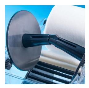
Care must be taken when replacing the fleece roll – please ensure the O-rings on the left and right side of the new roll are mounted in the correct way - see the arrow on the figure at the left. These O – rings prevent the roll from turning freely - this keeps the fleece always taut.
