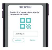
**2.** Now select the "New cartridge" option in Typus. You can then scan the QR code or enter the ID of the cartridge in the text field.
