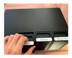
1. Remove the used cartridge from the Korallenwächter by pulling it out to the front. Remove the sealing plugs from the new cartridge and use them to seal the used cartridge. Caution! Always remove the orange sealing plugs first so that the pressure can escape. Place put a kitchen towel underneath for safety.
