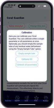
You can then start the calibration. Calibration runs automatically and takes approx. 30-45 minutes. The reference is almost completely used up.
